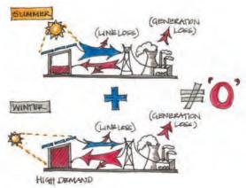
Figure 3. Source energy accounts for generation and transmission losses, but site energy does not.
